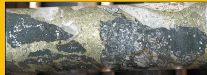
Tourmaline-chalcopryrite-cemented breccia. PALSUL13; 730m @ 3.58% Cu (from 66m)
